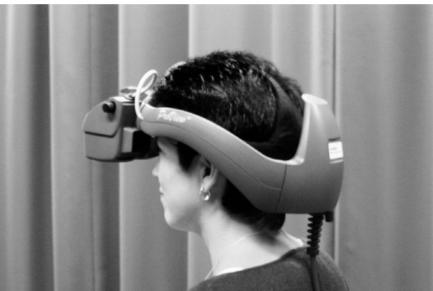
Abbildung 5: Head-Mounted Display ProView XL 50
